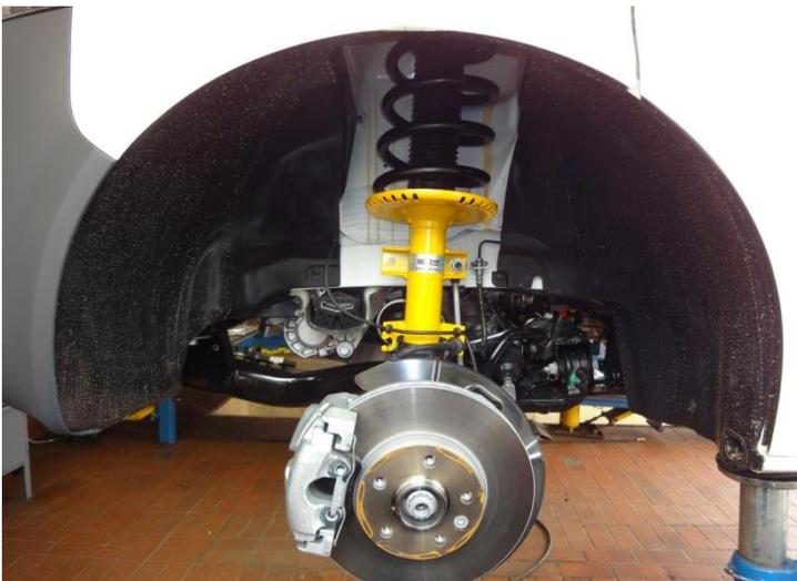
The mounting of the suspension strut is done in the reverse sequence of the dismantling. Insert the suspension strut up to the limit stop (possibly, remove rust on the contact surface before) and tighten from above.
