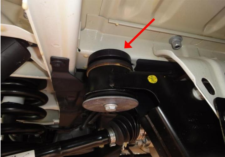
Mount the aluminium washer 1012 0054 or SFT5 HA15H below the left rear-axle mounting point at the back in the direction of travel, as shown in the image. Tighten screw with 50 Nm and rotate 180° further.
