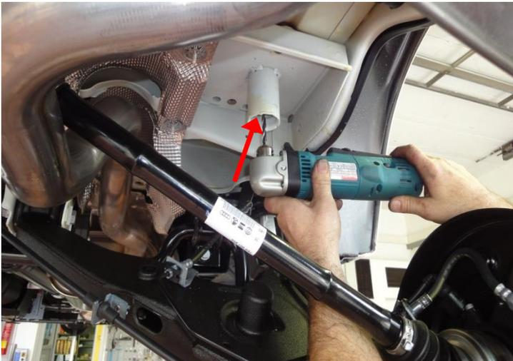
Enlarge the existing hole in the body with 7 mm drill (refer to image). Apply anti-corrosive coating after drilling.
