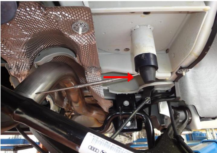
Press in the original buffer and with wire let the air pad above the buffer escape.
