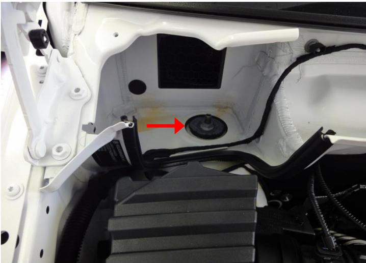
Remove plastic caps of shock absorbers on the front right and loosen nut on strut bearing until it is level with shock absorber piston rod.
