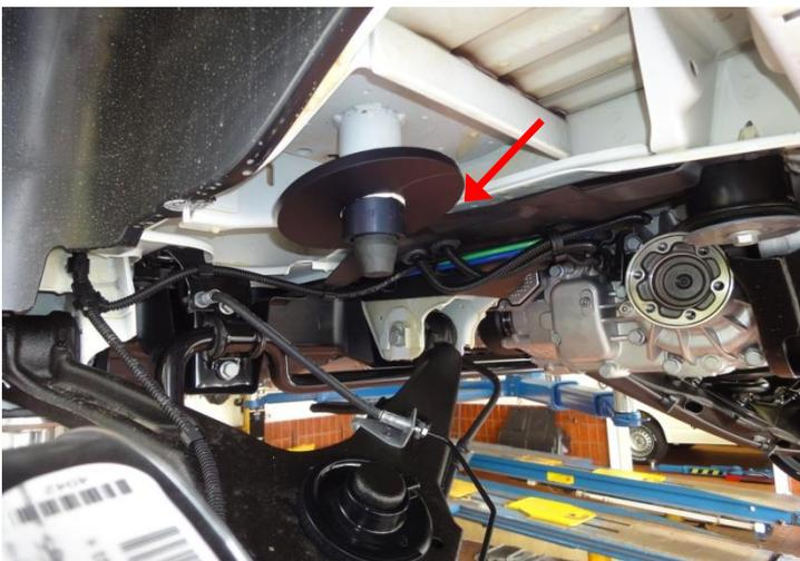
Insert spring pad 10mm or 15mm between body and upper rubber spring cap (if required). The pad is no standard delivery and is needed for special vehicle configuration, only.
