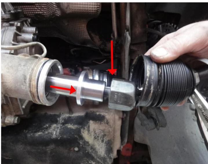
If optionally spacer washers for steering are supplied remove the left and the right steering rack gaiter and loosen the tie rod ball joints. Plug the supplied spacer washers with some grease onto the toothed rack and install again according the Volkswagen AG specifications.
