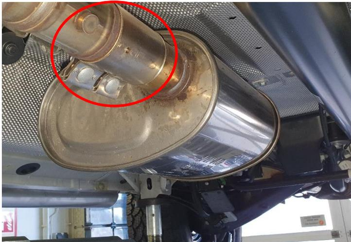
To be able to turn the rear exhaust pipe, the clamp in front of the center muffler must be loosened.
