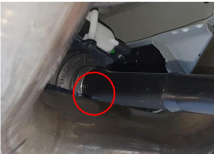
On vehicles manufactured as of MY 2021, it is possible that the right rear drive shaft – when fully extended – is in contact or almost in contact with the exhaust tract.
