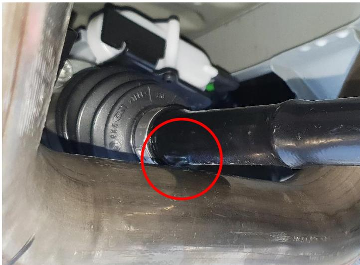
The rear exhaust train is now twisted so far that a distance between the drive shaft and the exhaust train of min. 5 mm is ensured.
