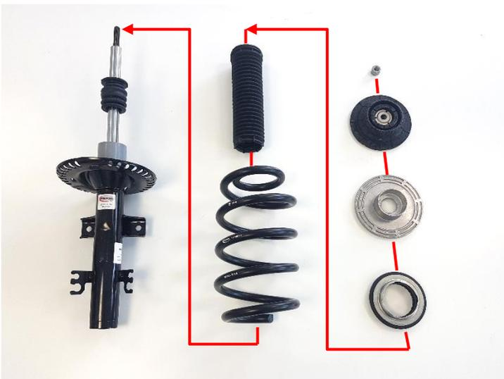
Assemble the new parts, shock absorber, spring and bump stop with the following parts from the vehicle, strut mount, aluminum spring disc thrust bearing and protective sleeve according to the order on the image. Finally, everything is screwed with the nut on the shock absorber and tightened according to factory specifications. (Image shows Monroe shock absorber, also applicable for red Koni shock absorber)
