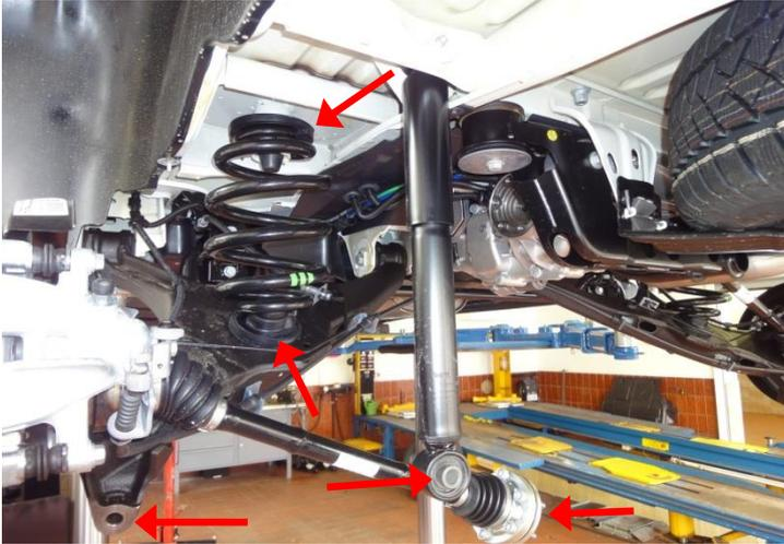
Completely unscrew shock absorber off its lower mounting (support rear axle lever with jack) and then loosen at the top. Release levers carefully and dismount spring, spring cap and buffer.
