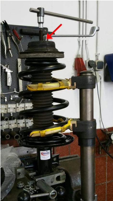
Loosen shock absorber nut and dismount spring. Note: Bellows will be re-used.
