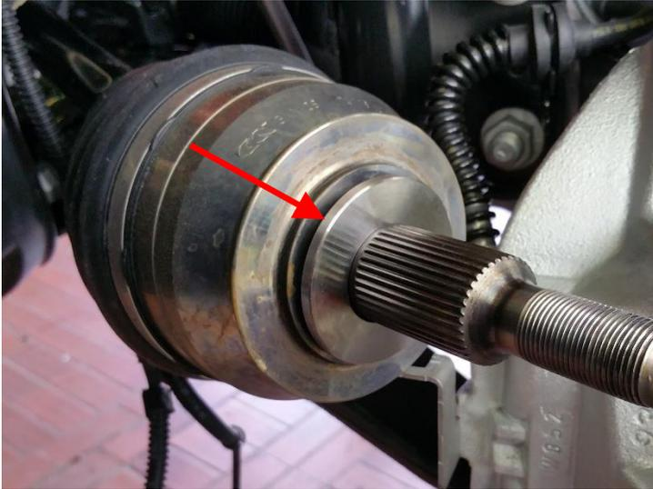
If the spacer washer 1014 0053 is supplied it has to be pushed across the stub axle of the front axle drive shaft with the flat continuous side to the outside.
