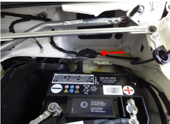
Remove plastic caps of shock absorbers on the front left and loosen nut on strut bearing until it is level with shock absorber piston rod.
