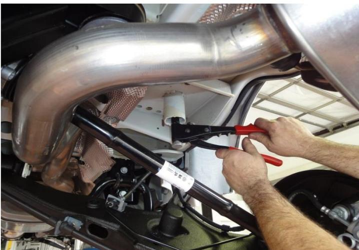
Insert 5 mm rivet nut using rivet pliers in the drilled hole.
