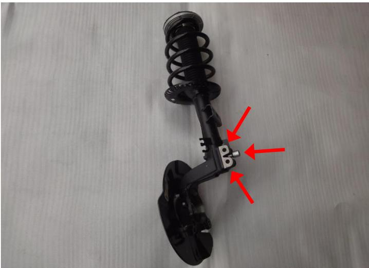
Loosen both the clamp screws on wheel carriers and dismount shock absorber with spreader.
