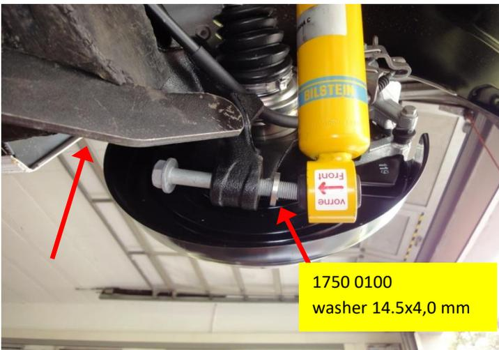
Fix shock absorber at the top, lift the trailing arm using the jack and screw the shock absorber with new screw and washer to the lower fixing eyelet. Pay attention to the mounting direction of the damper. Fix all the screws as per manufacturer's specifications.
