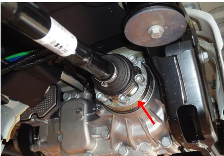
Completely unscrew drive shafts off the rear axle, left and right on the axle drive.
