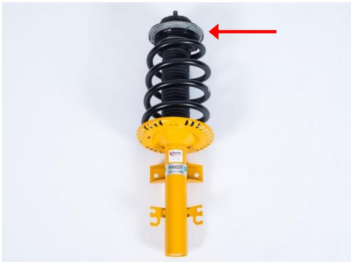
Place 13 mm spacer between aluminum spring disc and thrust bearing, as shown in the image.
