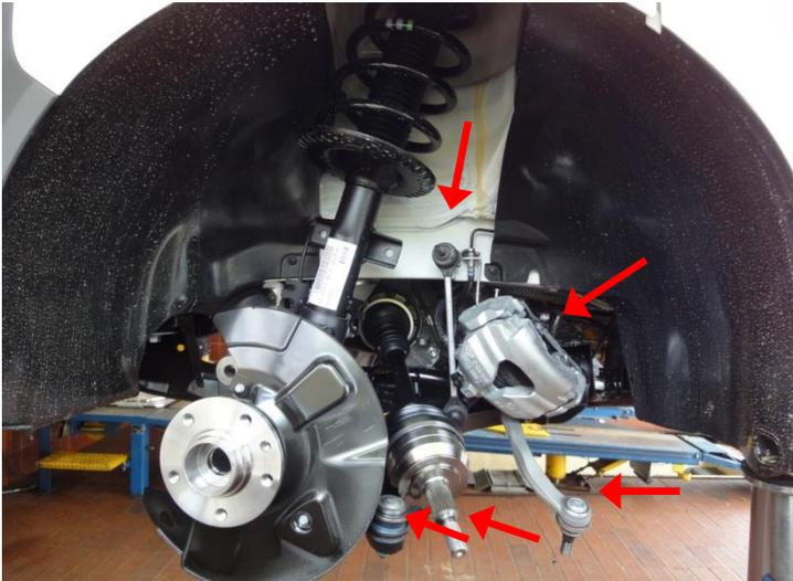
Loosen brake caliper completely with brake disc, steering link, stabiliser and ball joint, and pull suspension strut forward. Unscrew main nut of axle shaft and pull the shaft inward. Remove suspension strut from the wheel housing.
