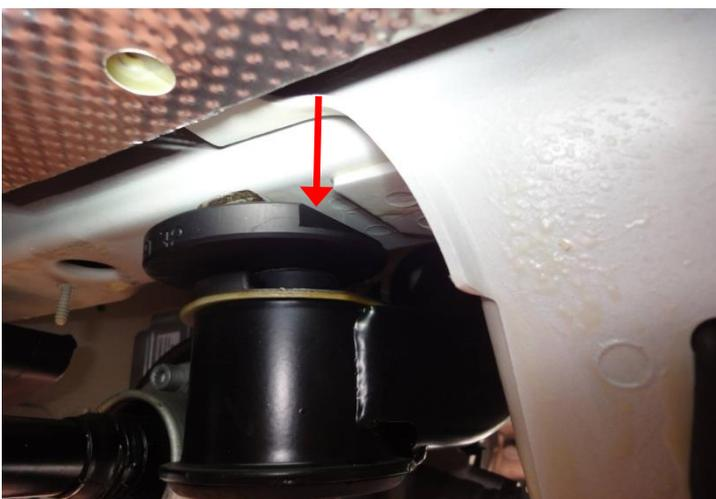
Support the subframe on rear axle gearbox with lever and loosen. Mount the aluminium washer 1012 0053 or SFT5HA15V with recess below the front rear-axle mounting point in the direction of travel, as shown in the image. Tighten screw with 90 Nm and rotate 180° further.
