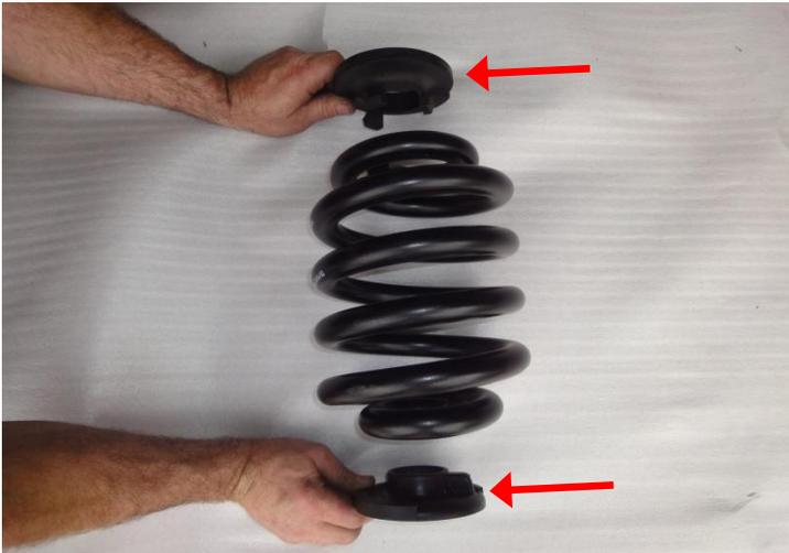
Spray both the rubber spring caps with silicon spray. Align the springs in such a way that the label is clearly legible, then attach the upper rubber spring cap 1012 0077 (Desert) or 1012 0085 (Desert HD and Maxi HD) to the spring at the top. Pre-position the lower rubber spring cap 1012 0076 (Desert) or 1012 0084 (Desert HD and Maxi HD) and mount with spring.
