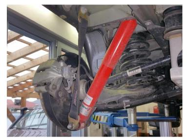
Put the rebound strap under tension and tighten the top as well as the bottom screw with 160 Nm.
