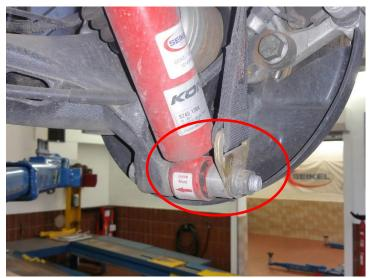
As done for the left side, assemble the rebound strap with the steel bushing and the supplied long collar screw below on the shock absorber.
