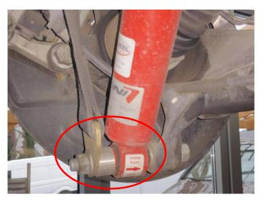
Replace the fastening screw of the shock absorber on the swing arm with the supplied 120-mm long collar screw. Behind the shock absorber, move the supplied steel spacer sleeve together with the rebound strap, as shown in the image, onto the collar screw and secure it with the M14 x 1.5 collar nut.
