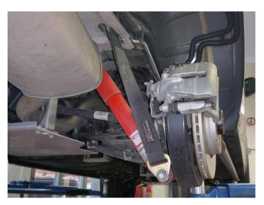
Put the rebound strap under tension and tighten the top as well as the bottom screw with 160 Nm.
