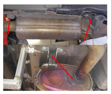
Loosen the rubber bearing of the rear and front silencer. Then disassemble the heat protection sheet and cut out the marked section.
