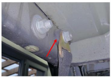
On the front screw, the black spacing sleeve (with the collar in the direction of the reinforcing plate), the rebound strap and the M14 x 1.5 collar nut are preassembled. The rear screw is preassembled with a washer and M14 x 1.5 collar nut.
