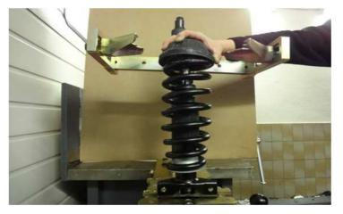
Disassemble suspension strut and replace spring. Coat contact surface of the spring at spring cap with anti-friction agent and complete suspension strut as per manufacturer's specifications.
