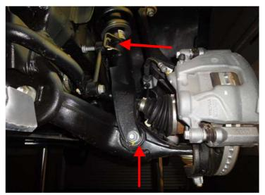
Loosen stabiliser on suspension strut and clamp screw on shock absorber at the bottom, lift out suspension strut completely.
