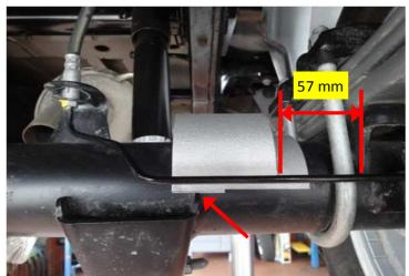
Place stop extension on rear axle tube and align to axle stop, as shown in the image. Stop extension must necessarily rest all over the axle body. Rework using garage tools, if necessary.
