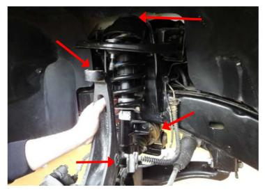
Tighten back the ball joint on the suspension wishbone at the top, mounting nut on the shock absorber at the top, drive shaft on front axle gearbox and brake pipe holder as per manufacturer's specifications.
