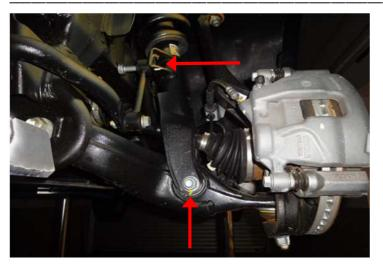
Tighten stabiliser on suspension strut and clamp screw on shock absorber at the bottom as per manufacturer's specifications.
