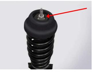
Insert nut with Loctite and tighten with 70 Nm. Only use nuts with 21 mm wrench width. <u>Note:</u>
