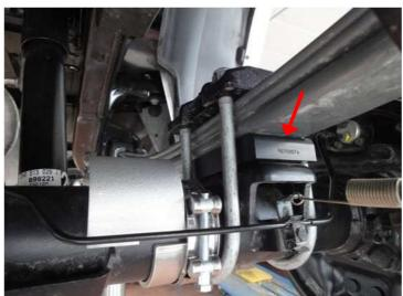
Lower the axle and lay spacer block of 25 mm rounding upwards. Lift axle and pay attention to the correct hub of the guiding bolt. Screw axle, leaf spring and spring tension plate with the new U-bolts and nuts provided. Replace shock absorber. Tightening torque as per manufacturer's specifications.
