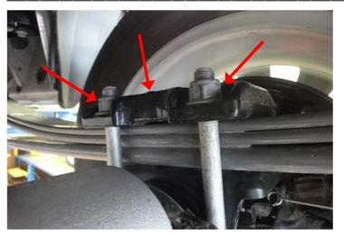
Dismount wheel and support rear axle with jack. Unscrew shock absorber at the bottom, unscrew four nuts on U-bolts and remove spring tension plate from the leaf spring.
