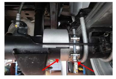
Slide the fastening clamp over the stop extension and half-shell and screw tightly.
