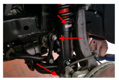
Tighten the stabilizer on the strut and the clamping screw at the bottom of the shock absorber as per the manufacturer's specifications.
