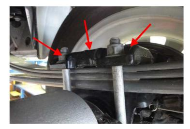
Remove wheel and support rear axle with jack. Unscrew the shock absorbers at the bottom, unscrew four nuts on the spring clip and remove the spring tension plate from the leaf spring.
