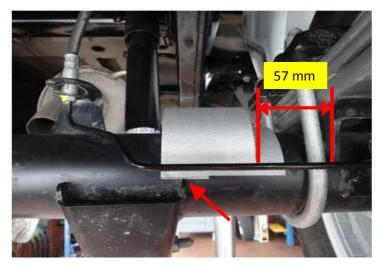
Place stop extension on rear axle tube and align to axle stop, as shown in the image. Stop extension must necessarily rest all over the axle body. Rework using garage tools, if necessary.
