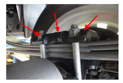
Dismount wheel and support rear axle with jack. Unscrew shock absorber at the bottom, unscrew four nuts on U-bolts and remove spring tension plate from the leaf spring.
