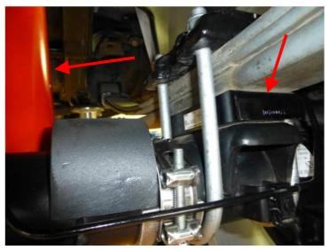
Lower the axle and lay spacer block of 25 mm rounding upwards. Lift axle and pay attention to the correct hub of the guiding bolt. Screw axle, leaf spring and spring tension plate with the new U-bolts and nuts provided. Replace shock absorber. Tightening torque as per manufacturer's specifications.
