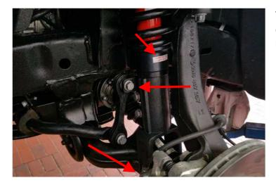
Tighten stabiliser on suspension strut and clamp screw on shock absorber at the bottom as per manufacturer's specifications.
