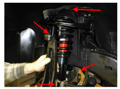
Install new Koni suspension struts provided in the delivery.
