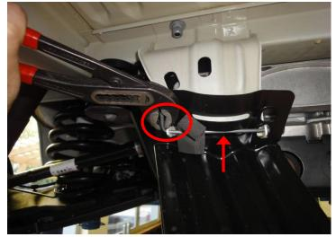
Bend open the pin as shown in the image and dismount latch fastener.
