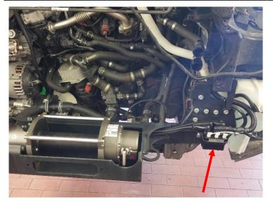
Fix the ECU for the winch pre-assembled with all the cables on the earlier iinstalled holder and connect the three thick cables to the cable winch, as described in the installation instructions of the cable winch.
