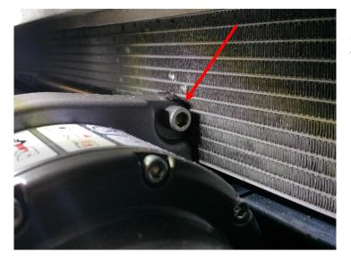
If the radiator is very tight on the winch, attach an abrasion protector, e.g. made of felt, to the winch to protect the radiator net.
