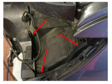
Lay the plus cable in the corrugated pipe below the headlight position towards left of fender and along the fender upwards to vehicle battery.
