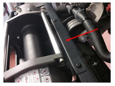
Fix the angle plate for cable routing supplied in the delivery behind the winch on the winch support with both the torx screws M6x10 supplied in the delivery. Tighten both the screws with 10 Nm.
