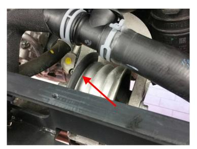
Fix the edge guard supplied in the delivery on the right plate edge of the front engine support.
