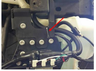
Fasten the earth cable of the ECU at the earthing point (--) on the vehicle frame.
