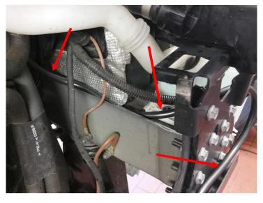
Fasten the earth cable at the earthing point (-), which is above the left vehicle frame as seen in the image.
