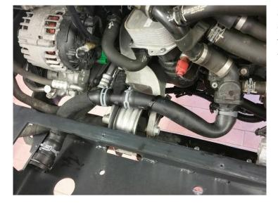
Separate the supplied and preassembled coolant hose on the coupling and replace the longer piece, as shown in the image, with the hose installed in the vehicle.
