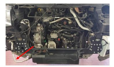
Fix the winch holder along with the left and right holder for the cooling pack on the frame heads. Use the 26 M8x35 hexagon screws and the M8 hexagon locking nuts supplied in the delivery for fixing.
