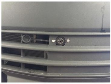
Cut the outline of the connector from the bumper and fit the bushing back on the bumper from inside.
