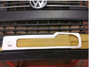
Mask the bumper in the area of marked surface with an adhesive tape and mark out the section for the cable fairlead onto the bumper using the stencil supplied in the delivery.
