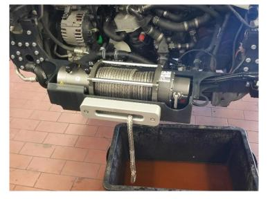
Fix the cable fairlead supplied in the delivery on the winch holder using the two countersunk head screws M10x40 and tighten with 35 Nm.
