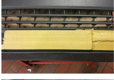
For connecting the remote control, mask the bumper as shown in the image.
