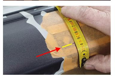
Remove the bumper from the vehicle again. Use a metal tape measure to mark two additional points vertically aligned 45 mm above the previously marked points.
