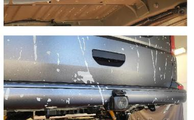
Fasten and tighten the trailer socket with the three supplied M5x35 pan head screws on the bracket plate of the towing bracket.
