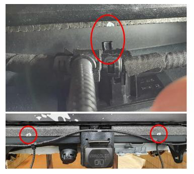
Before removing the provisionally mounted bumper from the vehicle, mark the points at which the two middle PDC sensors touch the filler pieces on the filler pieces.
