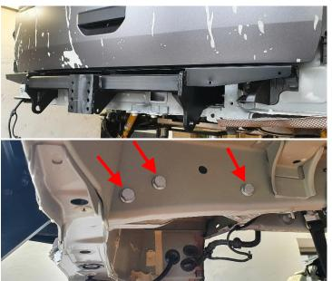
Insert the trailer hitch from the rear into the side members and fasten it to the side members on the left and right with 3 pcs M12x35 collar screw. Tighten the screws according to Volkswagen specifications for original trailer hitch (120 Nm).
