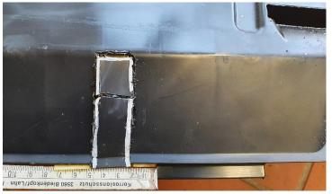
Make a cut-out on the underbody panelling in the rear area for the left towing point. As shown in the picture, this cut-out of 20 mm to 45 mm is to be made left-sided of the flap and to extend vertically up to the bend of the panelling.
