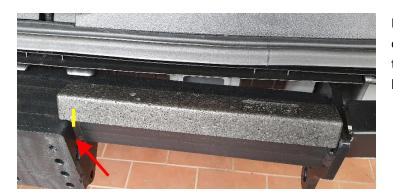
Place the two supplied foam filling pieces on left and right side of the square tube of towing bracket. Mark the overhang on the bolting bracket on the filling piece.
