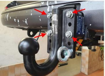
Fasten the hitch with screw plate to the Rockinger base plate using the four M10x45 socket head screws and four M10 collar nuts supplied. Tighten screws to 80 Nm.
