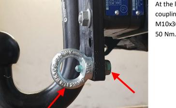
At the lowest mounting hole of the hitch coupling, fasten the M10 ring nut with M10x30 collar screw and tighten to 50 Nm.
