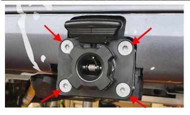
Fasten the Rockinger Varioblock to the trailer hitch with four M12x40 countersunk screws and four M12 collar nuts as shown in the illustration. Tighten screws to 80 Nm.
