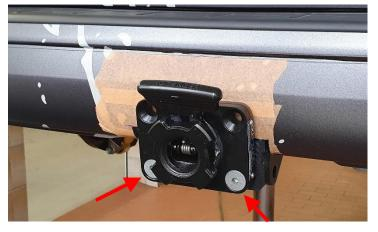
Place the bumper back on the vehicle. Then temporarily fasten the Rockinger Varioblock to the towing bracket with two M12x40 countersunk screws and two M12 collar nuts, as depicted.
