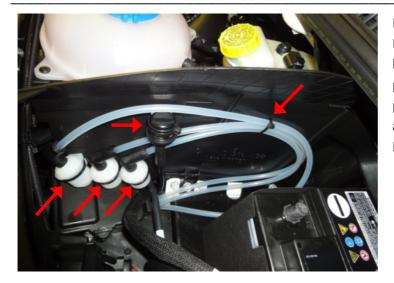
Remove the battery cover. Replace the original cover of the vehicle battery with the lateral cover with 4 filters provided in the delivery. Then attach the plastic pipes properly. Roll the PE pipes and secure with cable tie. Re-mount battery cover.
