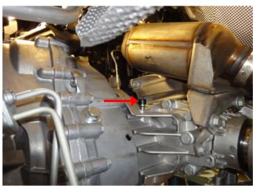
Remove the breather cap on angular gearbox and attach the other end of the pipe connected to the "Y" connector there.
