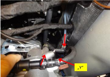
Connect pre-assembled pipe to manual gearbox using "Y" connector. From the "Y" connector, lay a PE pipe in the area of vehicle battery.
