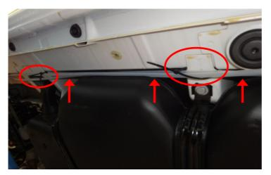
Lay 2 separate PE plastic pipes without any abrasion or kinking, as shown in the image.
