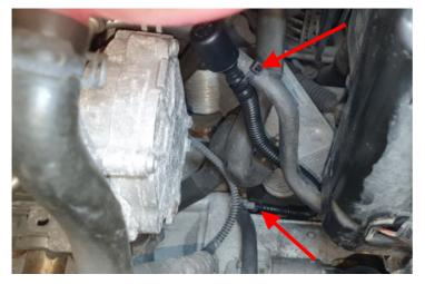
Pull off the vent cap from the DSG and attach the supplied corrugated hose, as depicted. Lead the hose up in the engine compartment and fasten it to the hydraulic line with a cable tie, as also shown in the picture.
