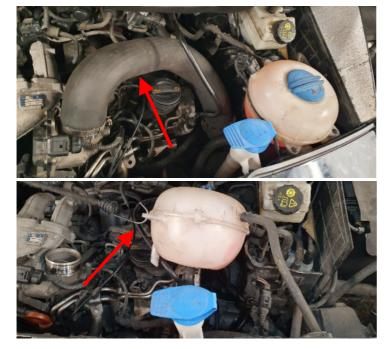
Venting of automatic (DSG) gearbox Remove the intake hose, loosen the cooling water tank and tie it to one side as shown in the second picture.
