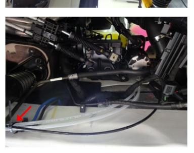
Bring all 3 pipes together and lay high up to the area of vehicle battery and secure.
