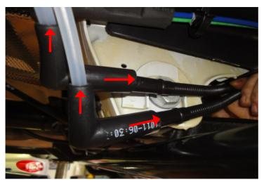
Connect 2 elbow connections, on the one side to the PE plastic pipes and on the other side to the original rear axle breather hoses. Then paste the intersections over the 4 heat-shrink tubings provided.
