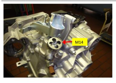
For vehicles up to MY 2009 (2,5 I TDI) remove breather caps on manual gearbox breather and mount retaining grooves in the connecting pipe using M14 external thread die.
