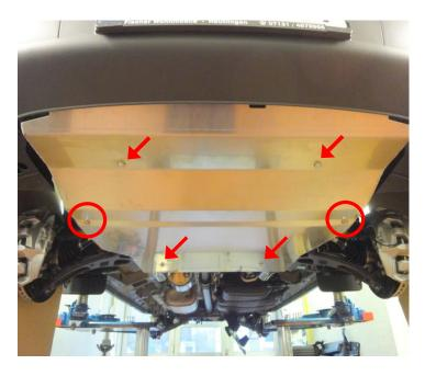
Fix engine protection to the original threaded inserts on the assembly carrier using 6 M8x50 screws.
