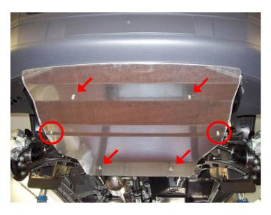
Fix engine protection to the original threaded inserts on the assembly carrier using 6 M8x50 screws.
