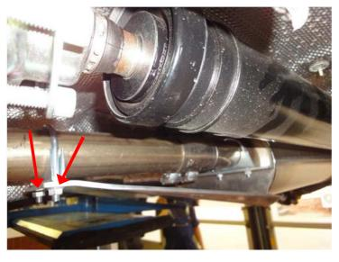
Fix protection plate with U-clamp at the front and 2 M8 nuts.
