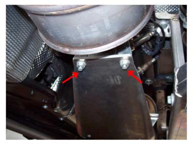
Cut the protruding thread of the front U-clamp by approx. 15 mm.
