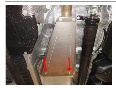
Fix protection plate with 2 M8 countersunk screws at the rear and align, tighten the countersunk screws with 15 Nm.
