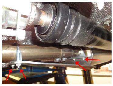
Likewise, tighten the 4 nuts of the U-clamps with 15 Nm.
