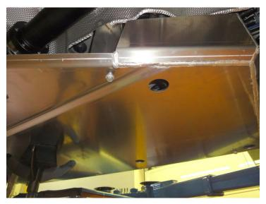
On the remaining 4 fixing points, fix the tank protection with 4 M8x30 screws and tighten with 30 Nm.
