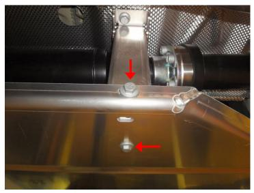
Fix tank protection with 4 screws M8x20 to both the brackets below the prop shaft.
