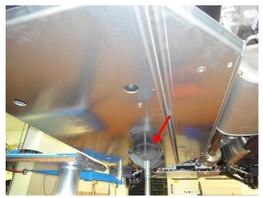
Unscrew the 4 set screws from the brackets and bring tank protection in position with the help of a gearbox lever.
