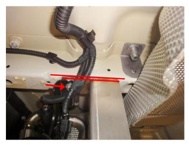
Fix bracket for traverse on existing screw and align parallel to bodywork reinforcement and tighten lightly.
