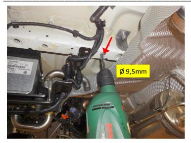
Remove the bracket again and drill a 9.5 mm hole at the indicated point.
