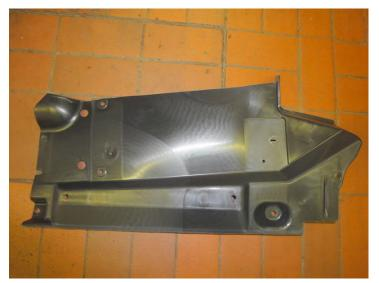
Mount the remaining centre body of the plastic cladding.
