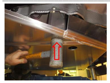
Using a soft-head hammer make 4 marks at the 4 lifting points from underneath the tank protection.
