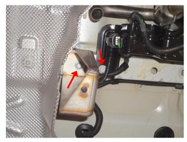
Fix bracket with M6x25 screws and tighten with 10 Nm. Tighten the original screw M8 with 30 Nm.
