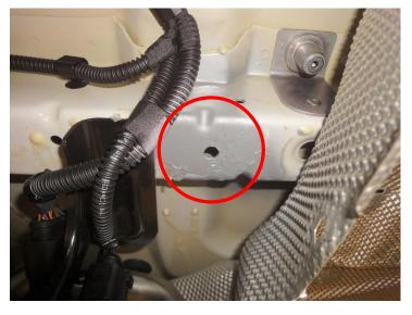
Remove rivet nut again, deburr drill hole and protect stress marks as well as traverse against rust.
