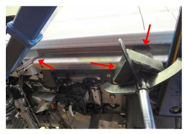
Firmly press the fastening rail on the car body before the drilling with the help of a wooden block and a gearbox lever.
