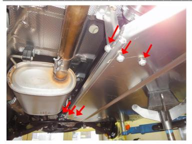
Fix the tank protection with 6 M8x20 screws on the middle bracket and tighten with 30 Nm.
