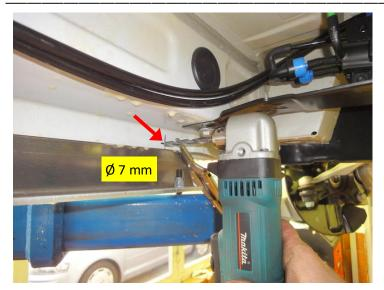
Drill all the points with a 7 mm drill through the side skirt and through the aluminium fastening rail.
