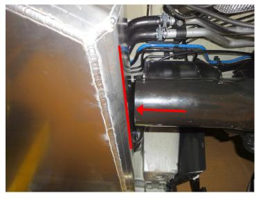
Push the tank protection back from the assembly carrier as much as possible.
