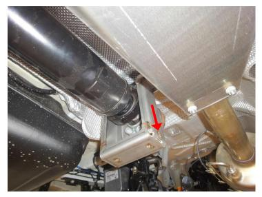
Assemble front bracket with threaded hole on the right, as shown in the image. Use two new M8x30 screws provided in the delivery and tighten with 35 Nm.
