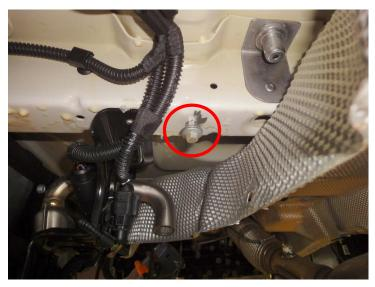
Fix hex collar screw M6 with hex rivet nut M6 and carefully hammer in the existing drill hole in order to expand it.
