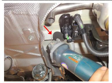
Remove existing set screw on traverse at front with angle grinder.
