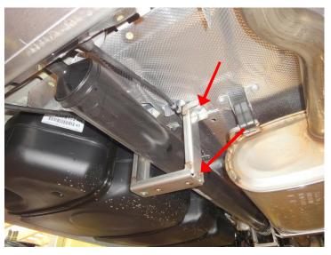
Assemble rear bracket with threaded hole on the right, as shown in the image. Use two new M8x30 screws provided in the delivery and tighten with 35 Nm.
