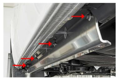
Tighten the fastening rail with 4 screws M6x25, flat washers and self-locking nuts with 10 Nm.
