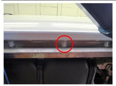
Mount fastening rail and centre with its recess on the middle of the three car body reinforcements. Finally, fix on the side skirt using a mole wrench.
