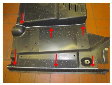
Mark plastic cladding as shown in the image and cut it.
