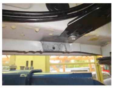
Deburr all the drill holes and treat with anti-corrosive protection.
