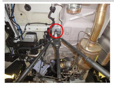
Insert rivet nut M6 with rivet pliers.
