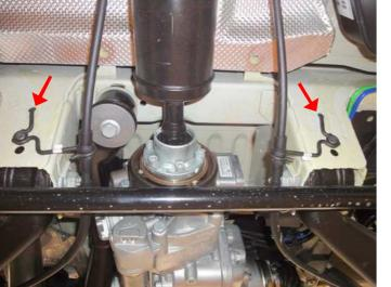
Remove both the hand brake rope holders on the left and right (are no longer required).
