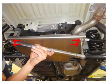
Fix protection plate at the back to the bracket that is still loose using 4 screws and M8x20 nuts and tighten with 30 Nm. Tighten rear bracket with 50 Nm and rotate 180° further.
