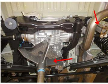
Support axle drive with gearbox jack and loosen rear axle drive fixings one after the other. Mount bracket with original screw (but do not tighten as yet).
