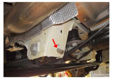
Spread the existing round hole on the left and right with 11 mm hexagonal tool.
