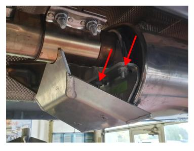
Align the protective plate horizontally on the middle silencer and tighten the 2 nuts of the U-clamp to 15 Nm as well.
