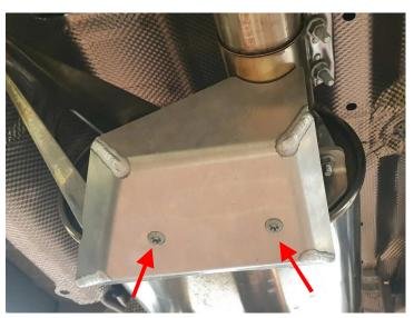
Attach the protective plate to the holder with 2 M8 countersunk screws and tighten them to 15 Nm.
