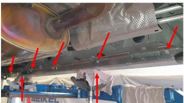
Using two transmission jacks, press the prepared Rockslider back onto the sill from below and fasten the terminal strip to the Rockslider from the inside of the sill using the M8x35 mm hexagon screws provided.
