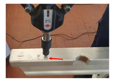
Insert an M8 riveting nut into all holes of the Rockslider.
