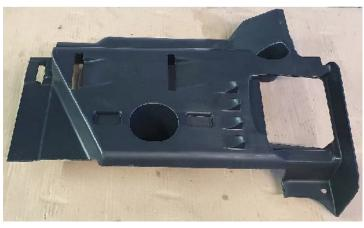
After trimming, clean and deburr the cut edge. Then mount the cladding again on the vehicle.
