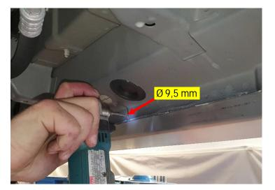
Drill all 5 marks with a 9.5 mm drill through the seam on the sill and through the Rockslider. Then remove the Rockslider from the vehicle.
