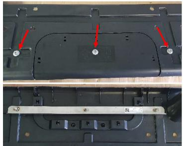
Fasten the reinforcing bracket with the three M6x20 screws supplied, as shown in the pictures on the left. Tighten the screws with 10 Nm.
