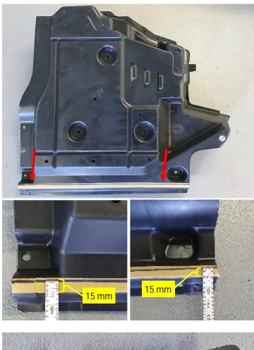
Trimming of the plastic claddings on T5 and T6: (T6.1 follows from page 15)
