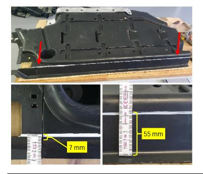
Mark and cut the <u>plastic cladding on the</u> <u>front right side</u>, see the pictures.
