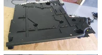
Mark and cut the <u>plastic cladding in the</u> <u>rear left side</u> as shown in the pictures.
