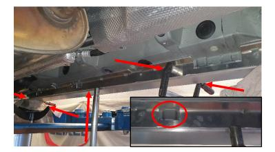
Place the right terminal strip from the inside against the seam of the sill and centre the recesses in the terminal strip using the body reinforcements. To fix the terminal strip, press it from below against the sill with a transmission jack and press it against the seam of the sill with two screw clamps together with the Rockslider.
