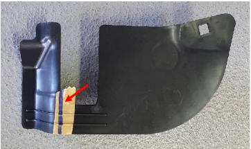
Mark the cover of the jacking point on the front left side as shown in the picture, cut it to size and clean and deburr the cut edge. Then mount the cladding again on the vehicle.
