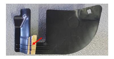
Mark the cover of the jacking point on the front right side as shown in the picture, cut it to size and clean and deburr the cut edge.
