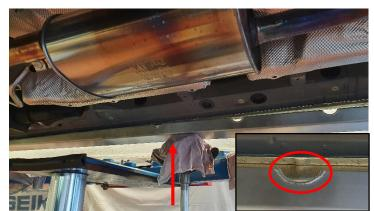
Place the right Rockslider from below on the right sill and centre the recesses on the 3 body reinforcements. Then press the Rockslider onto the body with a transmission jack.
