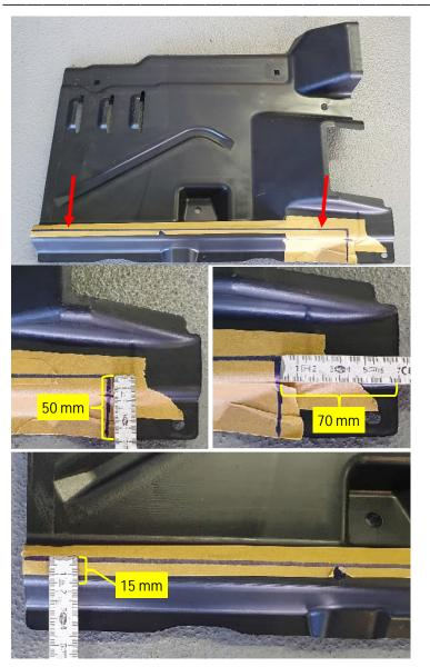
Mark the <u>plastic cladding in the rear on</u> <u>the right</u> as shown in the pictures, cut it to size and clean and deburr the cut edge.
