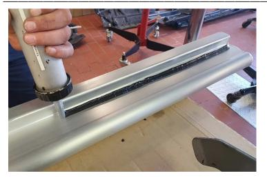
Before installing the Rockslider, a bead of car body sealant must be applied over the entire length of the top of the Rockslider profile, as shown in the picture.
