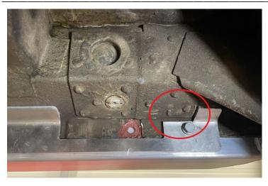
On vehicles with an additional reinforcement plate at the rear of the inner sill, the clamping strip must be reworked accordingly using workshop materials, as shown in the picture.
