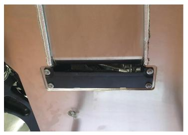
Finally, insert the air duct into the the protective plate and tighten it with the 4 M6x25 collar screws supplied.
