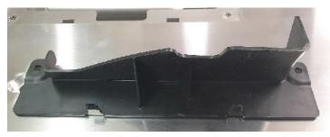
Dismantle the engine's sound insulation pan installed on the vehicle and remove the air duct shown in the picture on the left.
