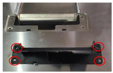
Drill out the two marked positions and the existing holes to  $\emptyset$  10 mm. Then clean and deburr the holes.
