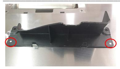
These are now the marks for the two missing holes on the air guide.
