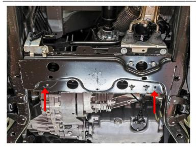
... and the rear two marked threaded inserts to the vehicle.
