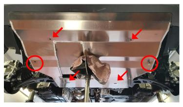
Screw the engine guard to the original threaded inserts on the engine mount using 6 M8x50 collar screws.
