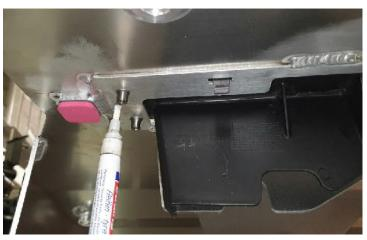
From the opposite side of the protective plate, transfer the position on the air guide through the two rear rivet nuts.
