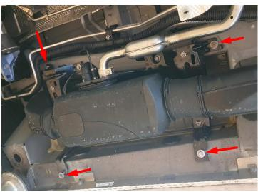
On vehicles with auxiliary air heating, loosen the four fastening screws of the holder for the auxiliary air heating marked in the picture by approx. 4 to 5 mm.
