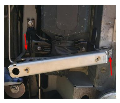
Slide holder 1, as shown in the picture, under the two front loosened screws of the parking heater holder.
