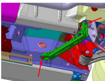
Install the supplied holder 4 as shown in the picture and fasten it with the M6 x 25 screw supplied and the previously removed M8 screw.
