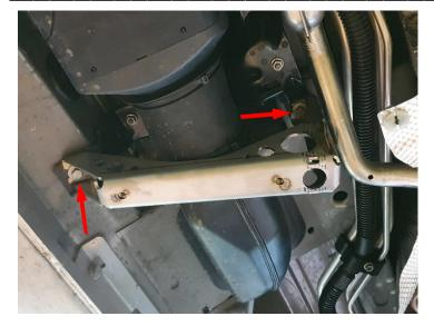
Slide holder 2, as shown in the picture, under the two rear loosened screws of the parking heater holder.
