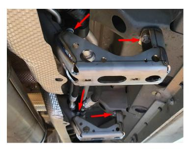
If present, loosen and remove the two cylinder head screws in the holders of the lines for the auxiliary air conditioning system.
