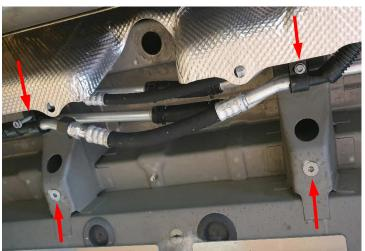
In the rear area of the right underbody, rivet nuts must be inserted at the two body reinforcements shown in the picture. The necessary holes are already present in the body.
