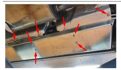
All 14 screws are to be tightened with 10 Nm of torque.
