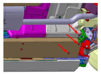
In the case of the protection plate for vehicles with a long wheelbase, three additional M6 x 25 screws are used for fastening to holder 4 and the rear heat protection plate.
