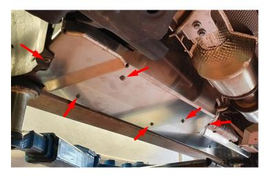
When installing the protection plate supplied, make sure that the heat protection plate of the exhaust system overlaps with the protection plate from the outside. The same applies to the front right wheel arch liner.
