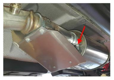
Align the protective plate horizontally on the middle silencer and tighten the two nuts of the U-clamp to 15 Nm as well.
