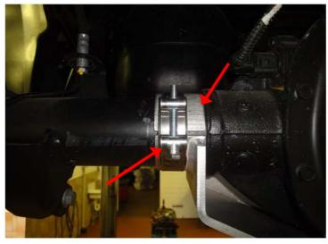
Place a half shell each on the rear axle pipe and position the band clamps in the centre.
