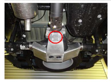
Fix protection plate to the suspension clamp using 4 M8x25 screws.
