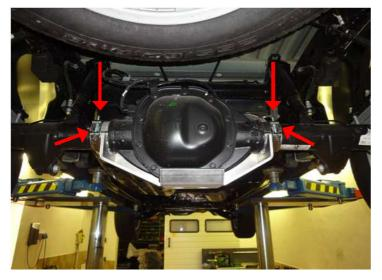
Align both the band clamps backwards. Tighten with 18 Nm.
