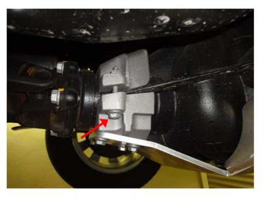
On the left side of driving direction, use a cylinder screw M8x70 with flange nut M8. Tighten all screws evenly with 15 Nm.
