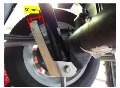
Adjust the distance from stone chip guard to shock absorber to 50 mm. Tighten lower shock absorber screw connection as per manufacturer's specifications.
