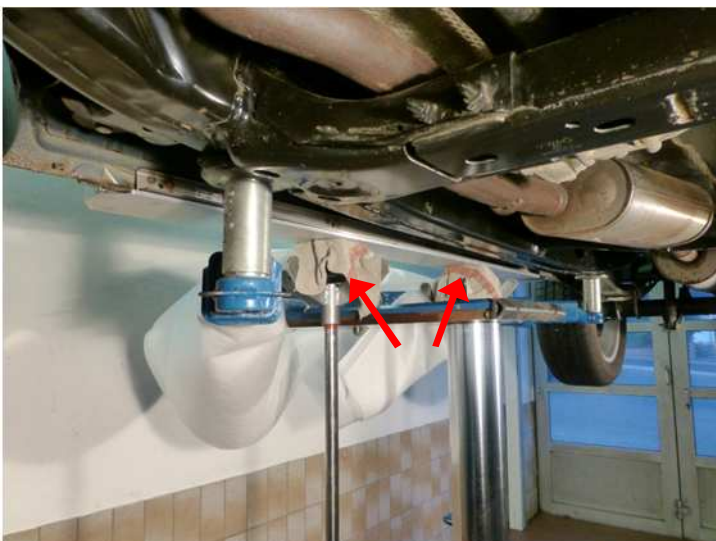
Press rock slider on the body using both gearbox jacks.
