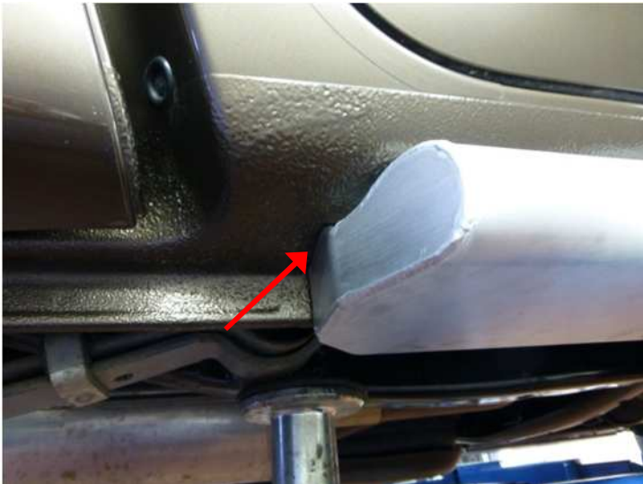
Installation position rear, align rock slider to contour line in the rocker.
