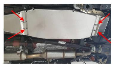
Secure the SEIKEL protective plate to the tank retaining straps with the four supplied M8 collar nuts and tighten according to the specifications of the vehicle manufacturer.
