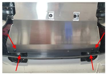
Fit the SEIKEL protective plate at the front of the towing brackets using both the two M10x35 bolts supplied and the M12 bolts previously removed and tighten according to the specifications of the vehicle manufacturer.
