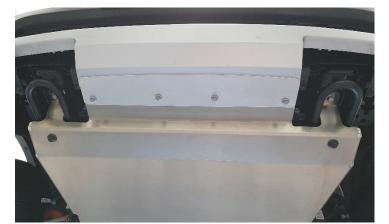
To do this, use the four supplied M5x25 screws, the washers and the M5 clamping nuts.
