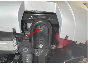
Mount the SEIKEL protection plate to the vehicle with the M10x35 bolts provided and tighten the bolts for the protection plates according to the specifications of the vehicle manufacturer.
