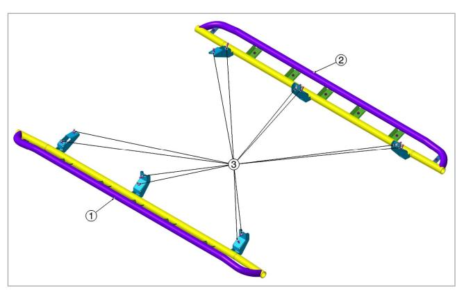
1 + 2 for Rockslider "Plus" two adjoining parts, welded
