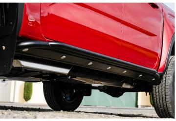
If the stone chip protection were ordered for the SEIKEL Rockslider, attach them on the left and right side using the countersink washers and M8x25 lens head screws provided and tighten them to 25 Nm.
