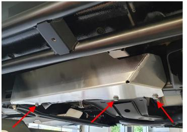
Secure the SEIKEL protective plate to the ladder frame with the supplied M10x35 and M8x35 screws and tighten the M10 screws to 50 Nm and the M8 screw to 25 Nm.
