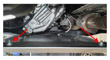
Place one of the supplied 11x34x3 washers on each of the M10x55 collar bolts at the top of the cross member and screw them in place with the M10 collar nuts.
