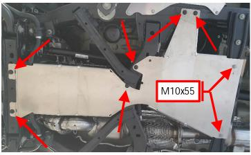
As shown in the picture, mount the supplied SEIKEL protective plate on the vehicle and fasten it with the supplied M10x35 collar bolts. The SEIKEL protective plate is fixed to the cross member in the middle of the vehicle with two M10x55 collar bolts each.
