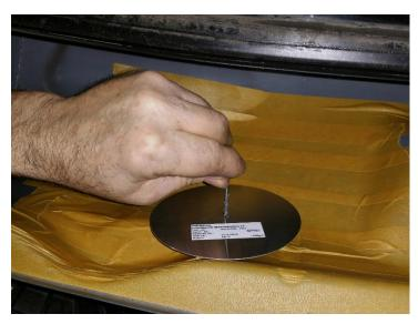
Fix the drilling template (2) provided in the delivery and mark the section for the breakthrough in waterbox on the intersection of both the earlier marked dimensions.
