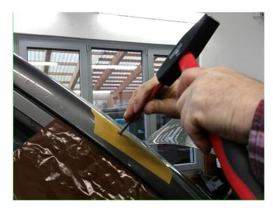
Remove the snorkel pipe again and with a drift punch, shape the inside panel of the A-pillar to the point where there is enough space for inserting the rivet nut.
