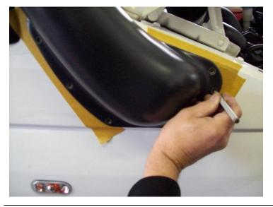
Join snorkel pipe and mark screw drill holes. Then drill the marked points to 7 mm.
