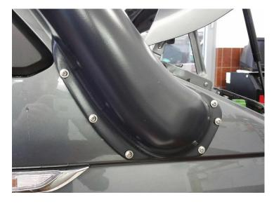
Fix the snorkel pipe to the fender using 6 lens head screws M6x20 and 6 collar nuts M6
