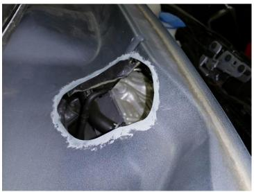
Deburr section and treat with anti-corrosive coating as per the specifications on page 2.
