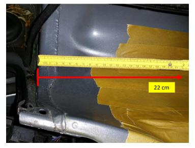
Measure, centre and mark the area of tube ducts.
