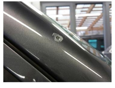
Insert rivet nut M6 in the A-pillar using rivet nut pliers.
