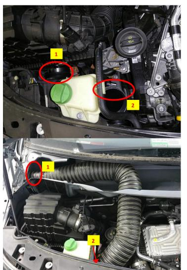
Dismount original suction pipe at "1" and mount the pre-assembled suction pipe provided in the delivery using the hose clamps provided in the delivery 100-120 mm ("1+2") on the air filter bottom part. If required, rework the connecting pipe of the pre-assembled suction pipe, so that it fits in the air filter housing without any problem.
