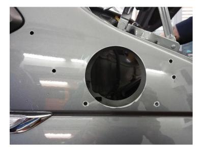
Deburr all edges, remove drilling chips and swarfs and treat against rust, as specified on page 2.
