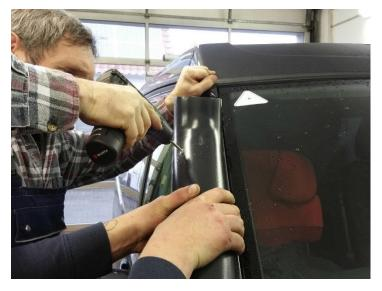
Press the snorkel pipe on the A-pillar and using a long 8 mm drill machine, drill through the already drilled hole in the air intake pipe in the A-pillar.
