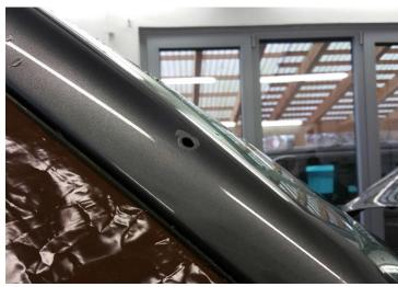
Deburr all edges, remove drilling chips and swarfs and treat against rust, as specified on page 2.
