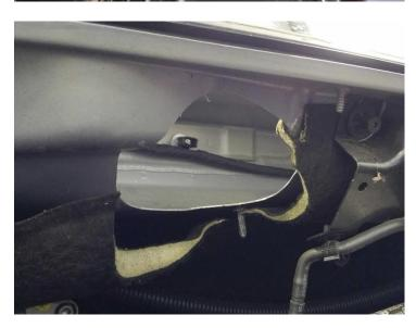
Cut the damping matting below the waterbox corresponding to the section.
