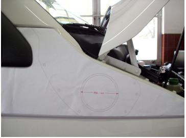
Mask the fender with adhesive tape to avoid scratches. Place the drill template for the air feed-through on the fender and align to the outline of the fender and fix.
