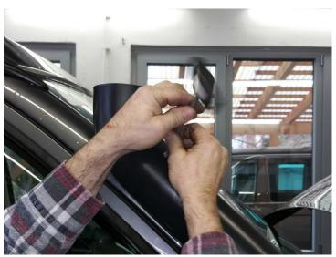
Insert the cylinder head screw M6x16 in the drill hole in snorkel pipe from inside and attach the snorkel pipe to the vehicle.
