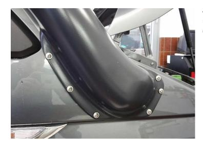
Align snorkel pipe to fender and temporarily mount using lens head screws M6x20 and 6 M6 nuts.
