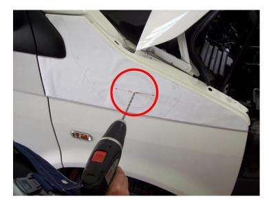
Mark the big section for the air feed-through on the fender, drill in the centre and extend to  $\emptyset$  110 mm. Also cut identical hole from the partition panel behind the fender, as seen in the image.
