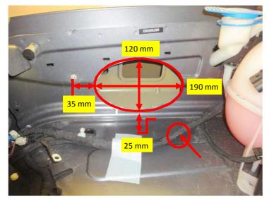
Mark section as shown in the image and cut it using hole saw. Remove excess wiring harness holder (arrow).
