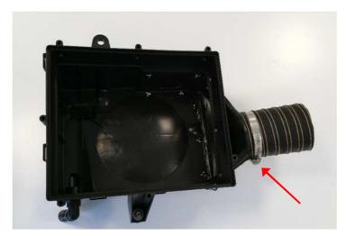
Fix hose fitting on the air filter housing at the bottom using the clamp provided in the delivery.
