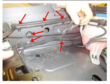
Loosen the wiring harness, earth strap as well as water hose in the engine compartment on the right and place aside.
