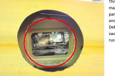
Through the fender breakthrough, mark the magnification on the engine compartment partition wall along the edge using a pencil, and cut it off.
