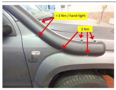
Tightening torque in Nm.
