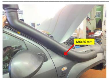
Align snorkel pipe to fender using 3x M6x20 and 1x M6x30 with washers and nuts. Screw in both the missing screws M6x20 mm in the rivet nuts, align snorkel pipe to A-pillar and tighten both the screws at the top.
