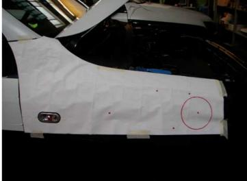
Place the drill template on the fender and align to the outline of the fender and fix. Using template, transfer all 4 screw holes and air pipe breakthrough onto fender. Make air pipe section (Ø 120 mm) and the 4 holes (Ø 7 mm).
