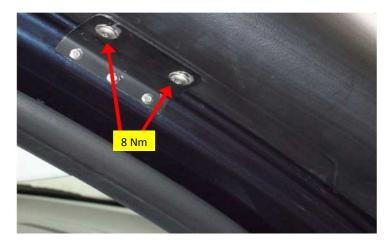
Screw the bracket with the pipe, do not completely tighten the screws as yet. Align bracket along the A-pillar and make three 3.2 mm drill holes for the blind rivets in the A-pillar. Preserve drill holes with anticorrosion agent!
