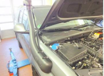
Fix both the air filter housings, mount all the hose connections back to their original points and complete the wheel house again on the right.
